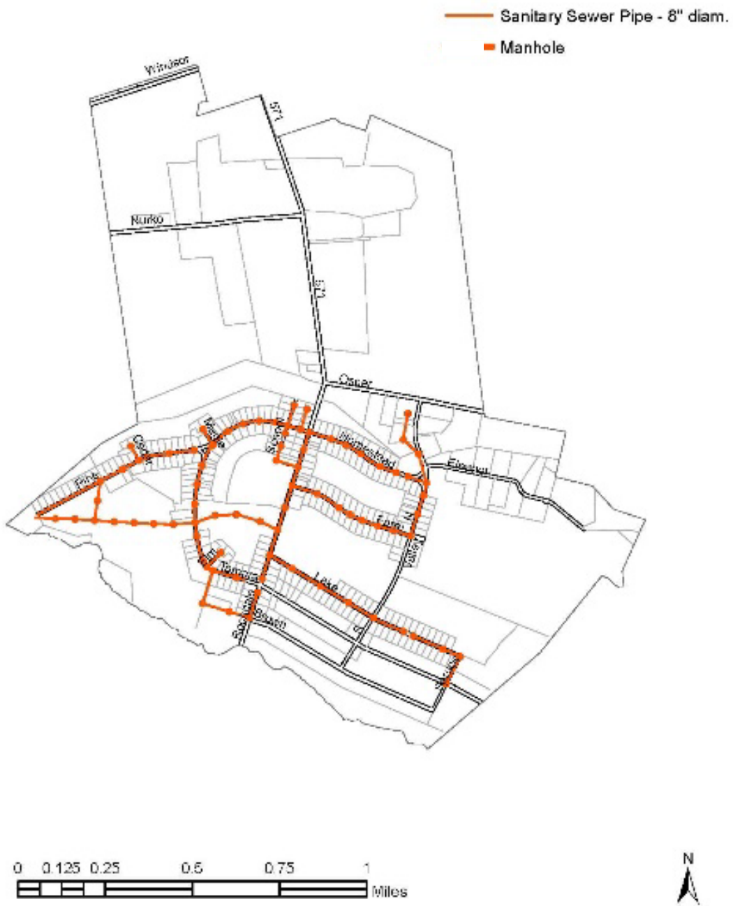
Map 10. Sanitary Sewer pipe distribution. (Derived from CAD drawing supplied by Roberts Engineering Group, LLC.)
